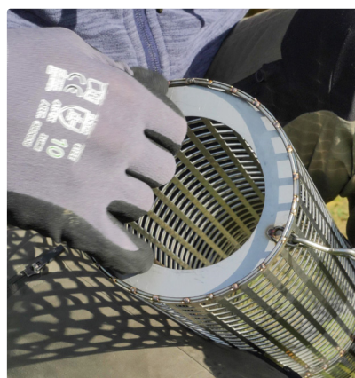
Place the tray inside the insulation pipe so that the chain sticks out through the topmost line of holes.
